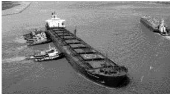
Several tugs assisting a vessel grounded just outside of a navigation channel.
