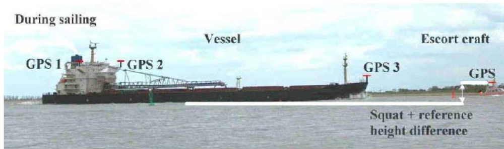
Fig. 2: Schematic presentation of the SHIPS - measuring method for dynamic conditions
