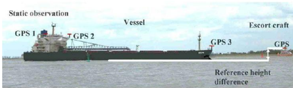
Fig. 1: Schematic representation of the SHIPS - measuring method for static conditions
