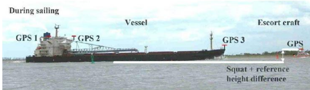
Fig. 2: Schematic presentation of the SHIPS - measuring method for dynamic conditions
