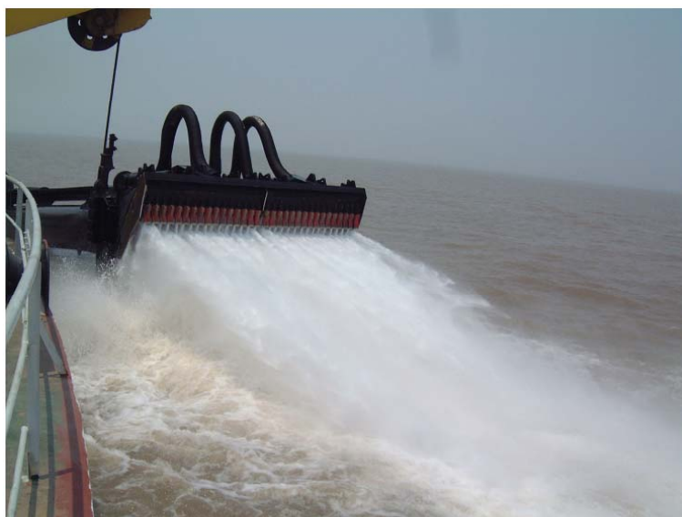
Fig. 8: The Wild Dragon® draghead showing its teeth and jetwater system.
