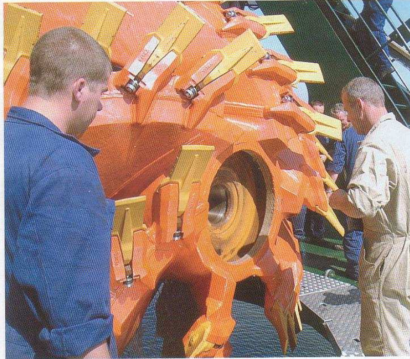
T8 cutter system just installed on d'Artagnan
