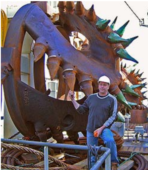
BIG TEETH: Due to extremely hard clay in the seabed, the JFJ de Nul's cutter, the world's largest, is working with an employed power of 4000 KW at the cutting head to open the 2 m deep and 10 m wide trench in one go.
