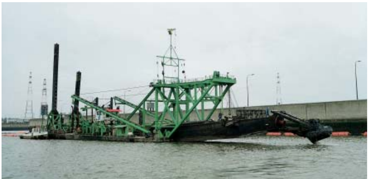
Figure 13. The scoophead reduces turbidity during dredging.
