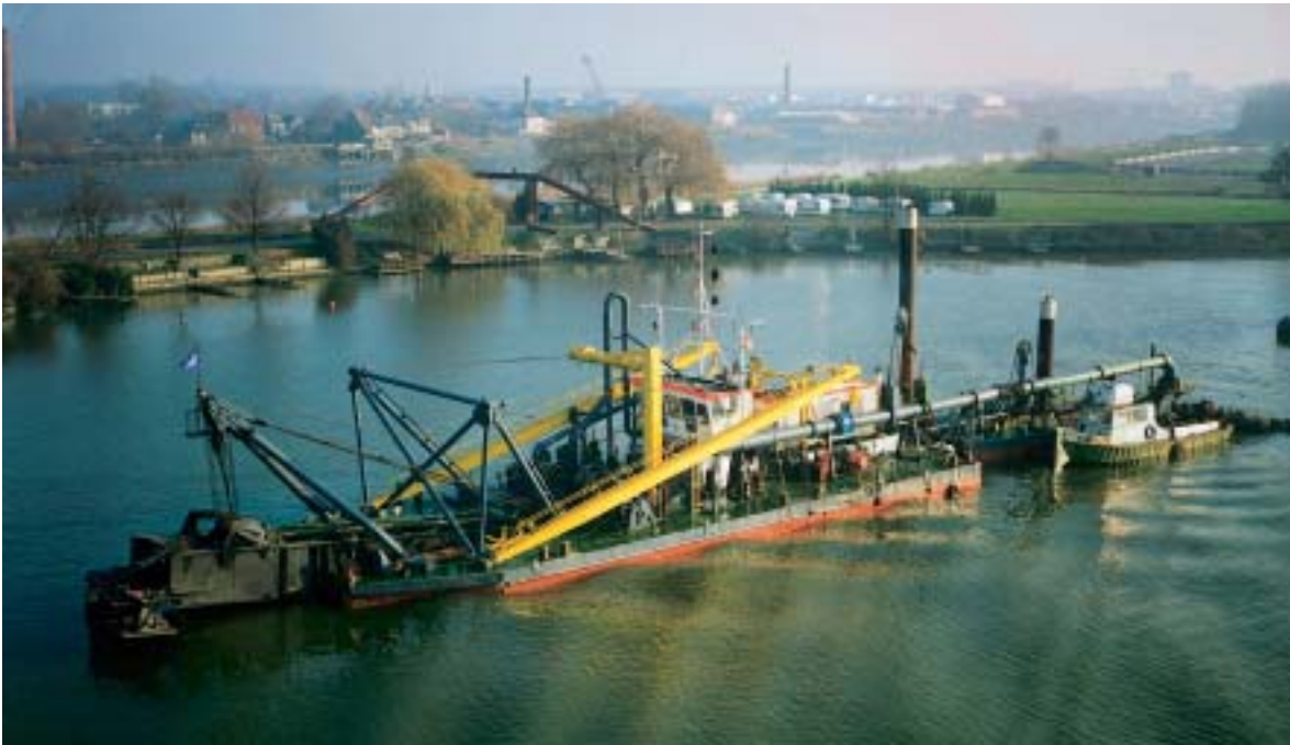
Figure 14. The cutter dredger Vlaanderen XV has been rebuilt with a sweephead, an environmentally friendly dredging system.
