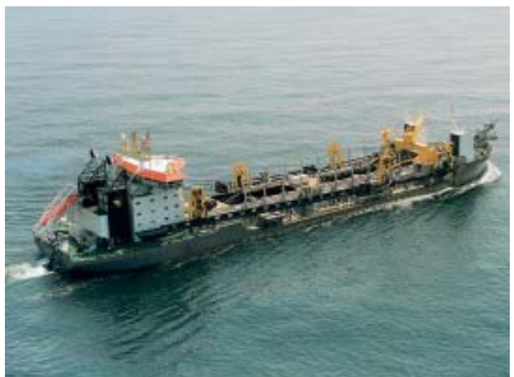
Figure 6. In June 1997 the WD Fairway became the world's largest trailer with a hopper capacity of 23,425 m 3 .
