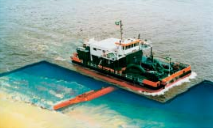
Figure 12. Through this artist's rendering underwater, the unique design of the water injection dredger Jetsed can be seen.
