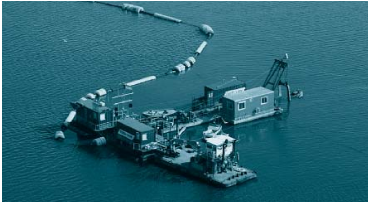
Figure 16. The closed auger, Willem Bever, has been used to dredge in highly contaminated waters.
