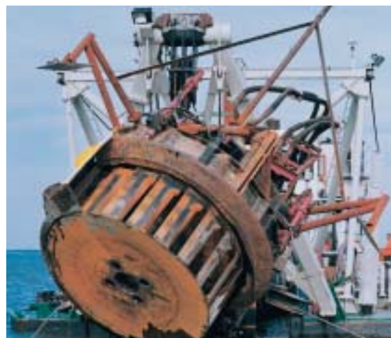
Figure 15. Close up of the environmental disc cutter installed on the Vecht .
