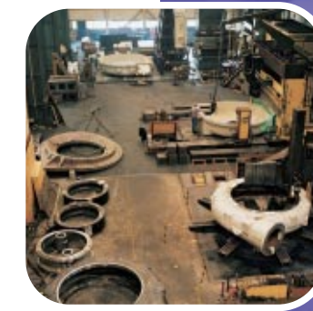
Machining includes computer controlled systems able to handle parts up to 12 x 4.5 meters to an accuracy of 0.01mm.
