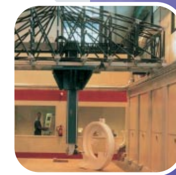
five axis computer controlled facilities means housing mould design at extraordinary accuracy.
