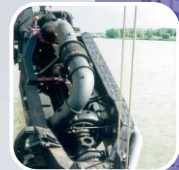
with submerged dredge pump on horizontal frame for easy access.
