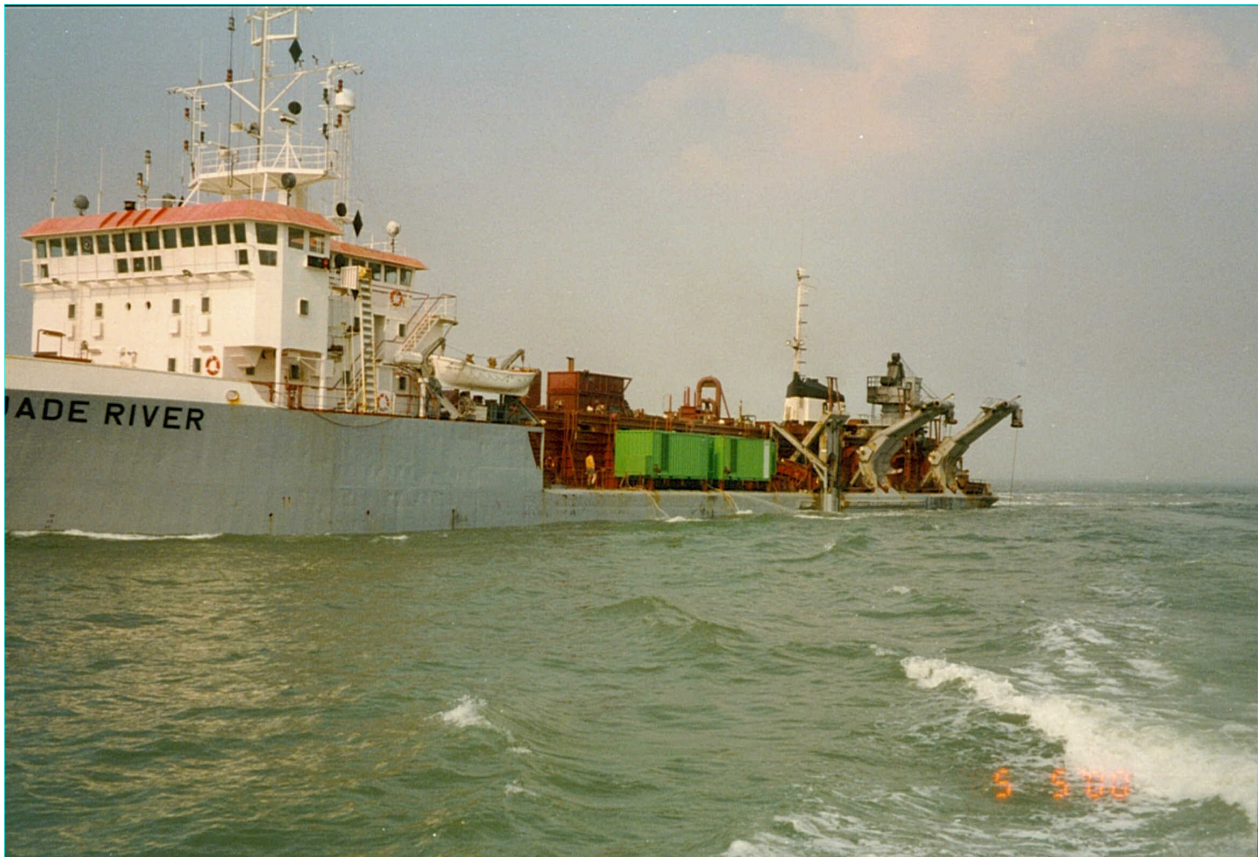
Fig 5: TSHD JADE RIVER with the high pressure pumps
