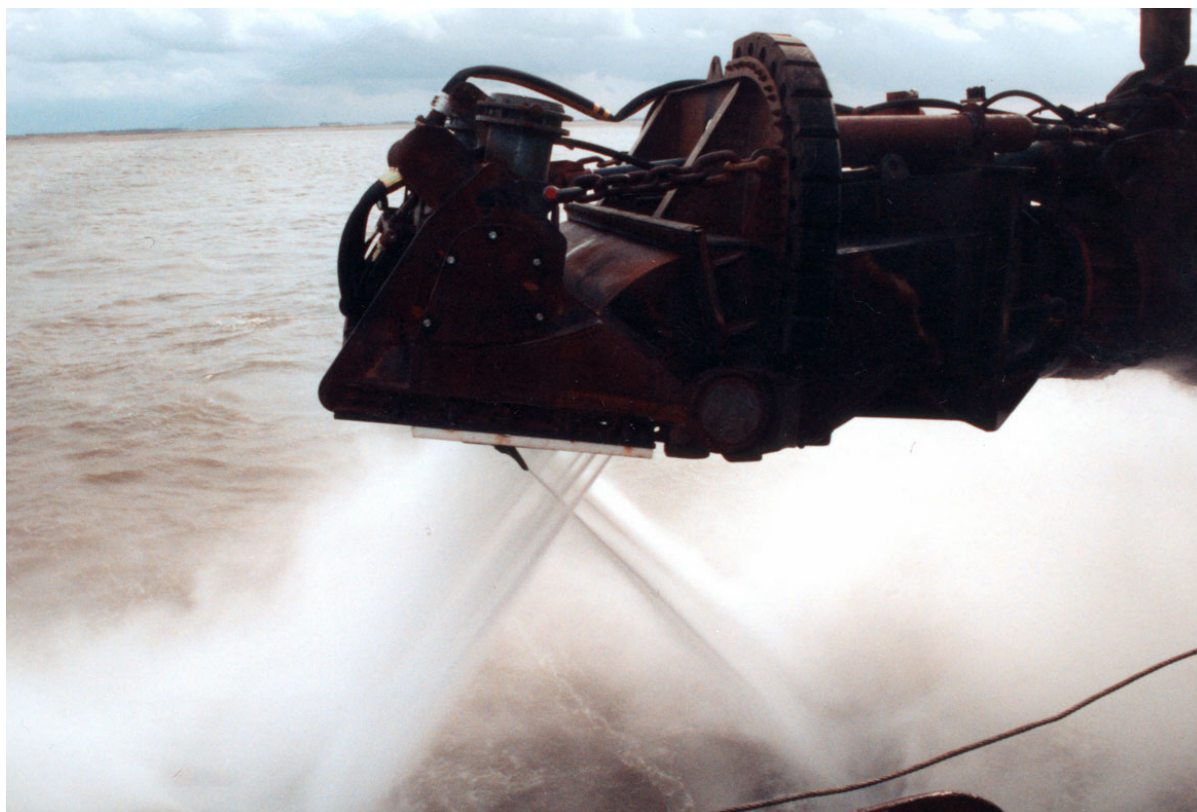
Fig 4: Picture of the DRACULA®-draghead on the TSHD JADE RIVER
