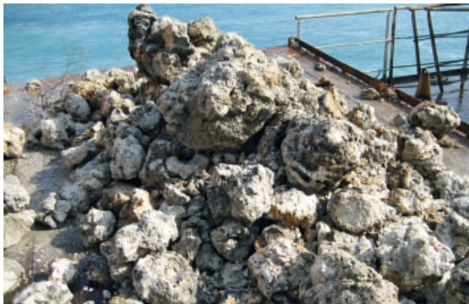
Figure 7. Coral blocks removed from the ripper draghead.
