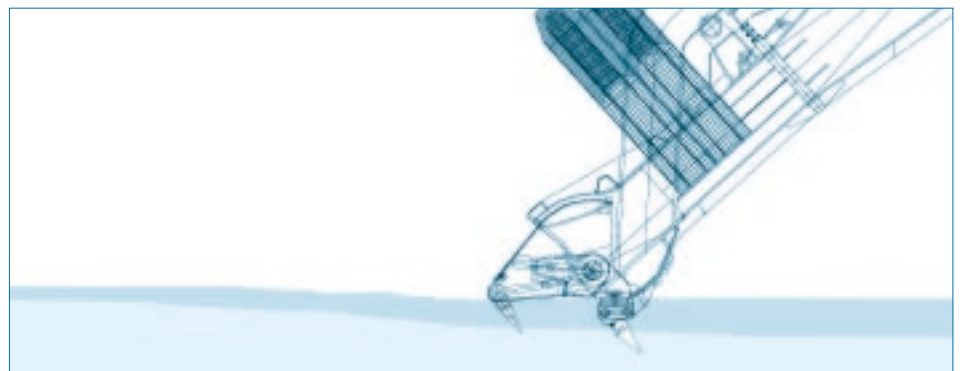
Figure 6. Drawing of draghead with ripper teeth on seabed.
