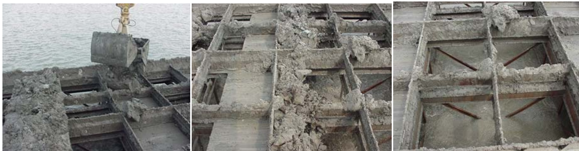
Figure 8: Midsection of the specialized rock dumping vessel
